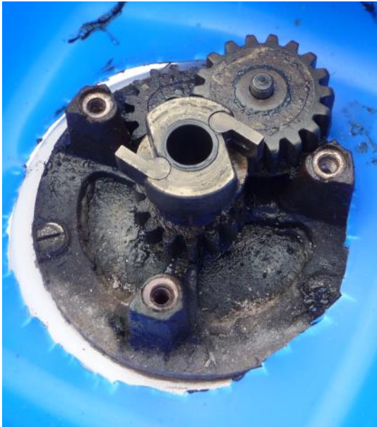
On this winch, the pawls will only go one way
