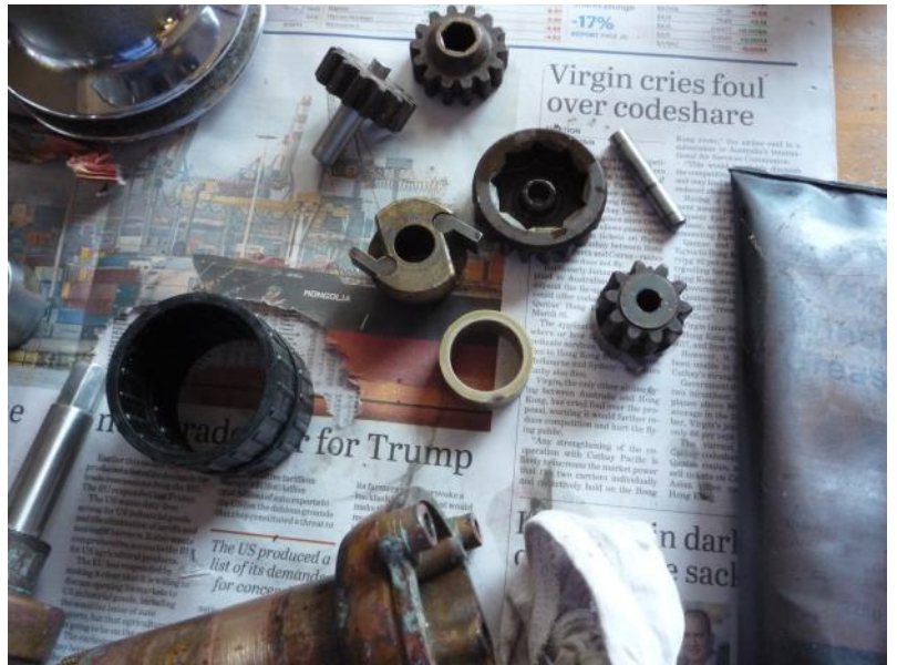
Cleaned parts ready for grease and reassembly...
