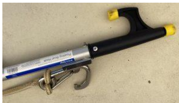
Another useful tool for snagging an incapacitated MOB is a mooring hook (Wichard makes a good one) attached to a pole or boat hook.
