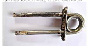
applied to it during retrieval, fine cracks can occur in the bedding compound as it ages. This allows the ingress of salt water through capillary action. This is not removed during wash-down. The variation in oxygen content, the next time it's wet with salt water, is sufficient to cause corrosion as the low oxygen area in the crevice becomes anodic. The protective Chromium Oxide surface film is attacked by chloride and it is unable to reform. However
